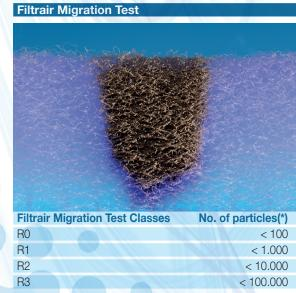
(\*) Number of particles larger than 10 microns per cubic meter counted on the clean air side
